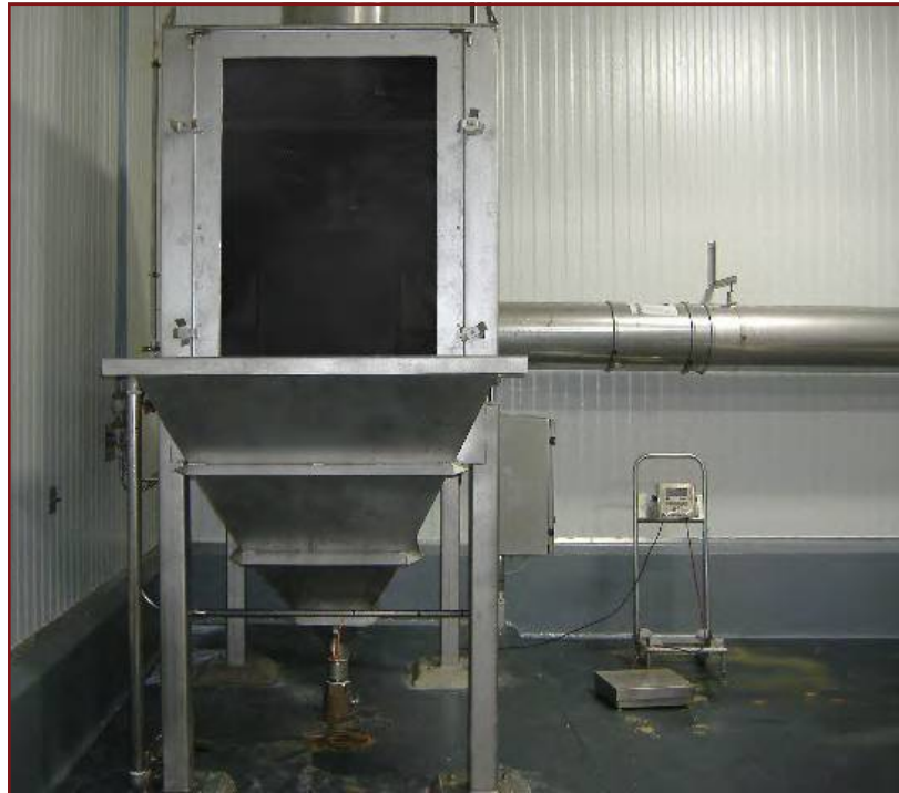
Stainless steel unit for spices with a fast acting ball valve for water flush Food processing
