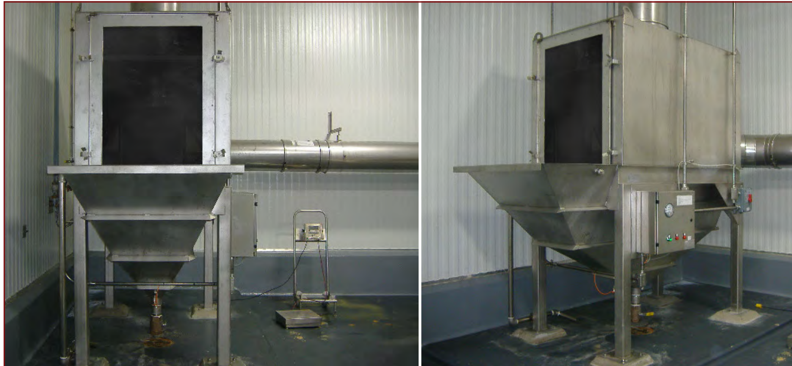
Stainless steel unit for spices with a fast acting ball valve for water flush Food processing
